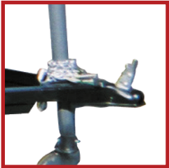
2" trailer hitch & heavy duty jack
