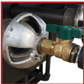
Air Mixer and Brass Gas Valve on the end of Burner
