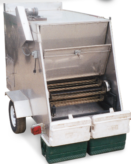
Model 306 shown in operational position while unloading corn into coolers.
