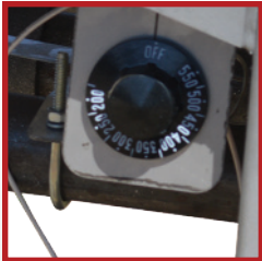
Gas valve & thermostat are both needed with the full hood
