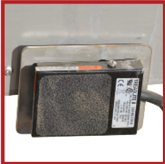
Foot switch for forward or reverse rack rotation
